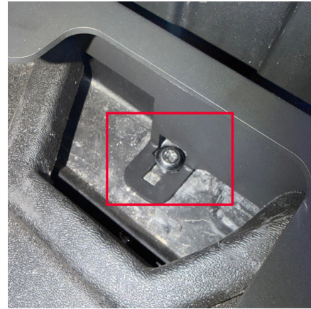
This mount uses the 2 factory T-40 bolts already installed on the bed. Remove and reinstall to hold the front of the mount to the bed.
