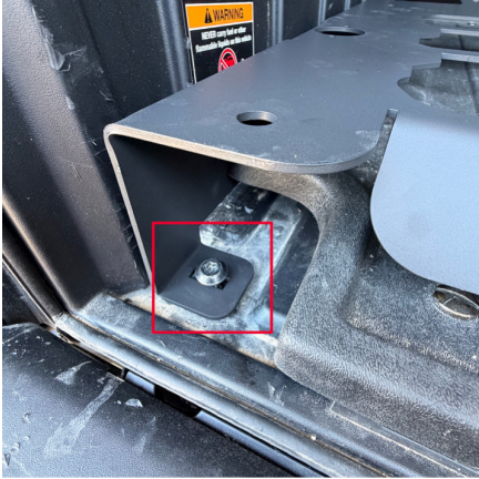
This mount uses the 2 factory T-40 bolts already installed on the bed. Remove and reinstall to hold the rear of the mount to the bed.
