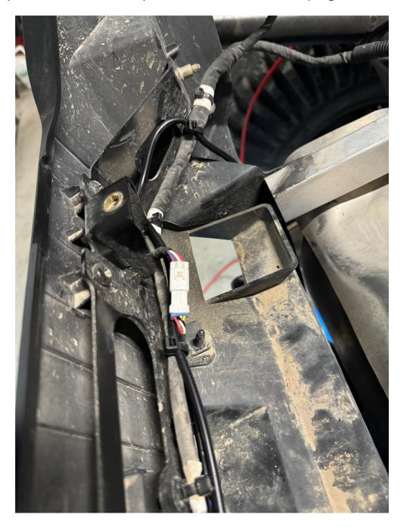
Step 3: Using the RUS Offroad Camera Relocation bracket as a template, drill 2 holes using a 5/16 drill bit.
