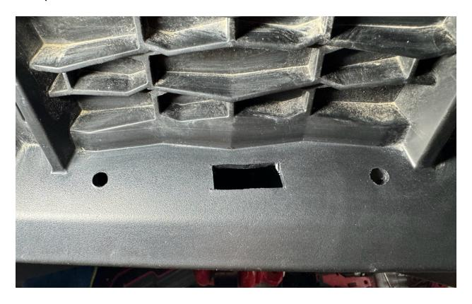
Step 4: Install the factory camera into the RUS Offroad Relocation Mount and install to RZR using the two plastic retainer clips. Be sure to feed the wire through the hole and up to the camera plug before mounting. Install top cover onto camera mount. Plug in camera to factory connection.
